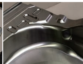
Cutting edge had normal wear without abnormal damage after finishing 7 hours of machining. Finished surface was much smoother and consistant versus competition.
