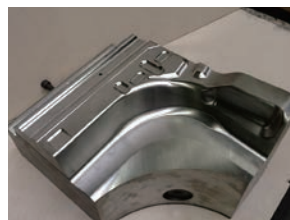
Cutting edge had normal wear without abnormal damage after finishing 7 hours of machining. Finished surface was much smoother and consistant versus competition.
